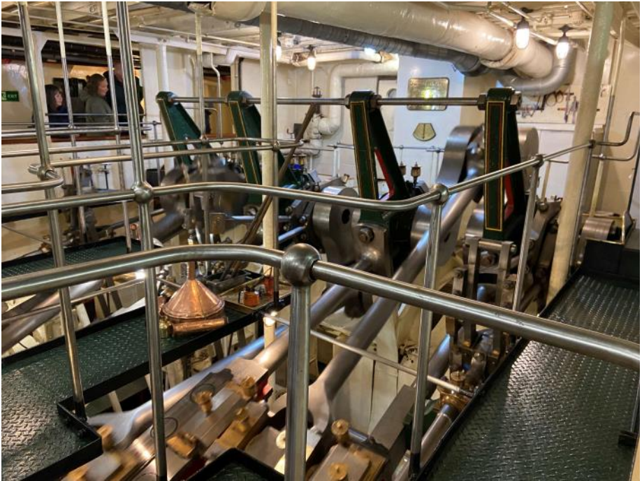
Waverley's triple expansion engine from the viewing gallery
